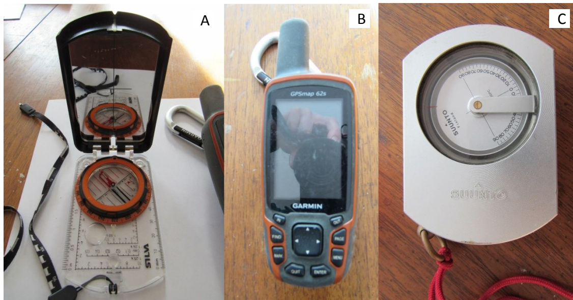
Figure 20. Equipment used in the location and description of the plots: A. mirror compass with declination set at about 14°W depending on the site, B. Garmin GPS mapping unit and C. Suunto manual clinometer.
